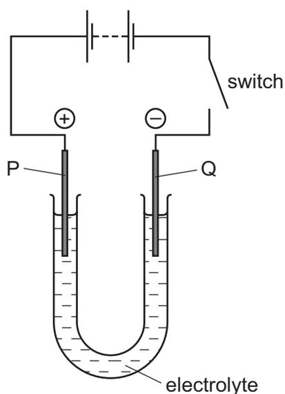
When the switch is closed, the solution around electrode P turns orange because a halogen is formed.
